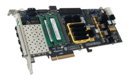
Figure 2.12: NetFPGA Board [65]
