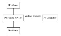
Figure 3.1: P4 Switch Architecture
