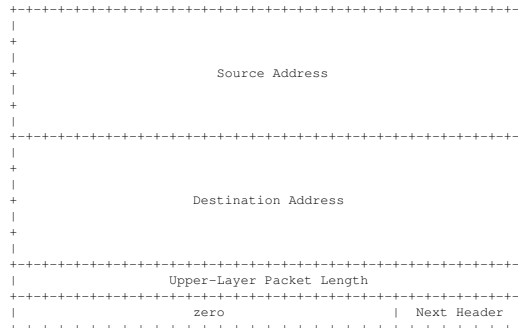
Figure 2.10: IPv6 Pseudo Header
